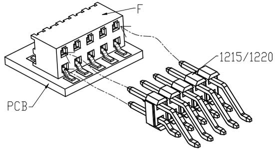
Allowed angular inclination tolerances, 5.0°
